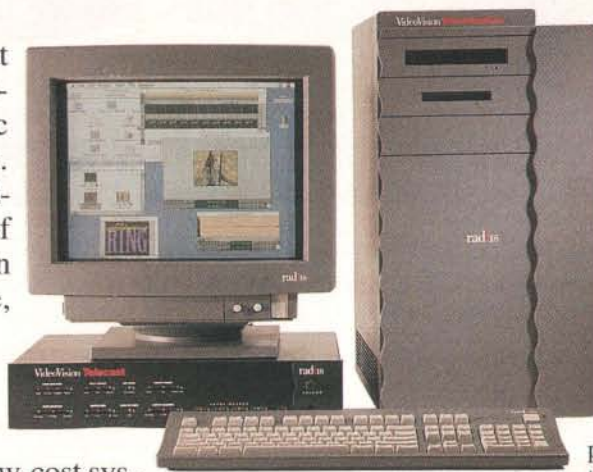
Radius's Mac OS-compatible systems will be high-end Macs for graphics or video-editing professionals. Radius's first systems will use the same motherboard as Apple's Power Mac 8100/110 and a PowerPC 601 CPU.
